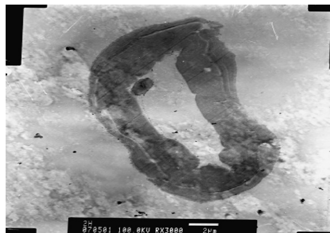
Fig. 8. Transverse section of wheat straw fiber after drying and rewetting.
